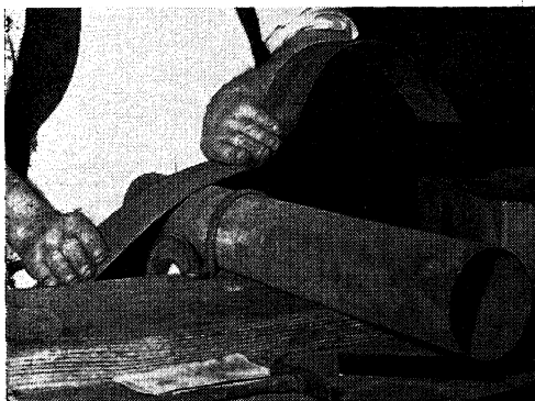
Showing how the guitar side is bent over the heated bending iron.
