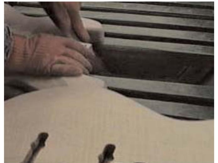
When the finish is dry, the bodies are moved on carts to the sanding area where they are prepared for the final finish. The top and backs are sanded on a stroke sander with between 320 and 400, and the sides are sanded on the end drum of a belt sander.
