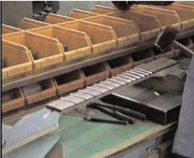
I first use the same radius as the fretboard to press the frets, and then I use a smaller radius to check the fret ends are pressed in. For example, if the radius is 9"
