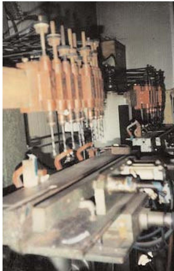
On areas that are bound such as the headstock, the binding is pre shaped in small presses that are the shape of the headstock and then the binding is installed, this saves the time of bending the exact shape for each headstock
