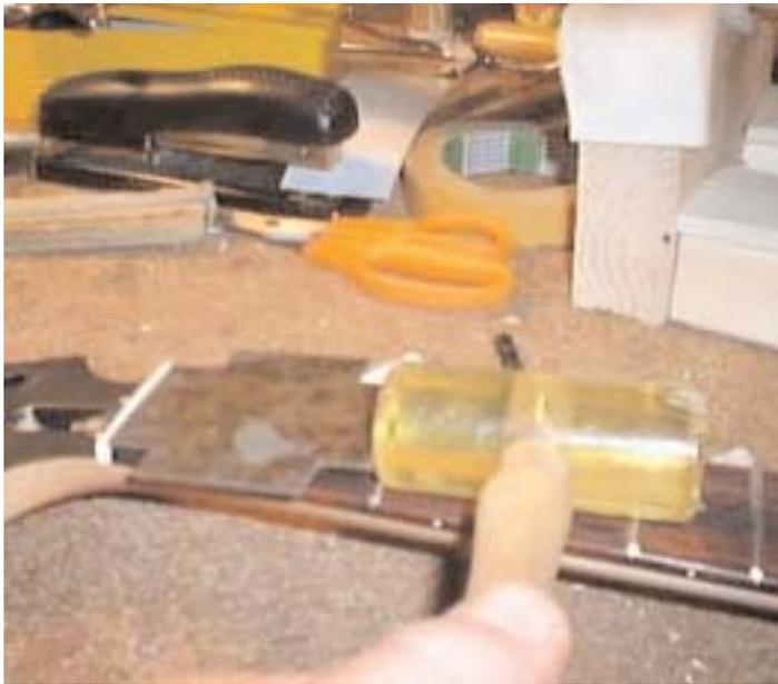
The next procedure is to remove the frets, be careful not to chip the wood around the fret tangs. The way I do this is to use a solder iron and rosin core solder used for wiring the electronics. I use the solder iron and actually melt the solder across the top of the fret.
