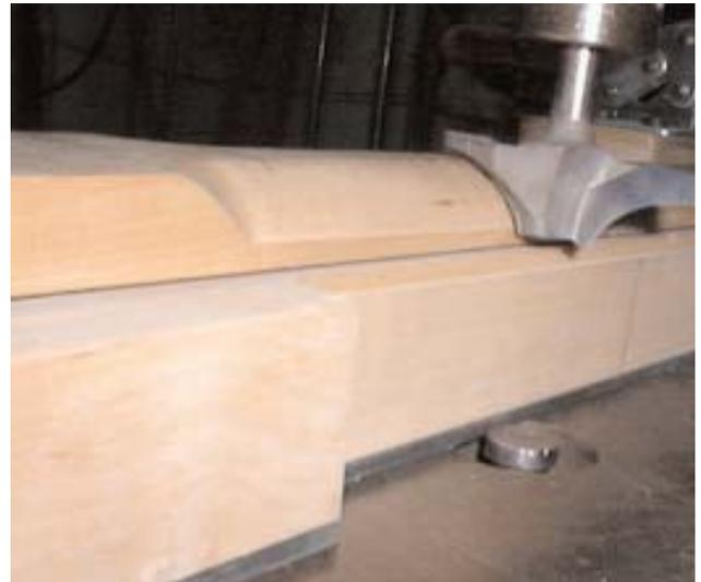
Now I want to shape the back of the neck; for this I also made a jig for the pin router. Depending on the neck thickness I use different shims to hold the neck up higher on the nut end of the neck. This holds the neck 2mm higher so that when I shape it on the pin router the neck will be shaped 2mm thinner at the nut area. If I did not have the pin router, I would rough shape the necks back radius on the belt sander.
