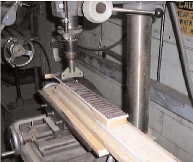
Now to install the frets I first use a rubber mallet to set the frets in the slots and then a drill press with the proper radius arbor to set the frets in. I made my own wooden presses a while back on my pin router but since I purchased the brass ones from Stew Mac, I have been using them.
