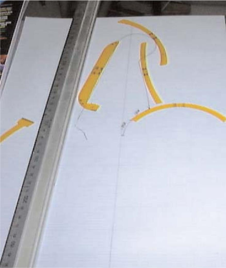
Start at a flat area like the neck pocket and work your way around the drawing, measure the distance from the center Line in Y and X and make a note; for example,  $X=-39.3$   $Y=28.71$  this is the start of the Arc; the Arc ends at  $X=-47.09$   $Y=40.38$  The radius between the two is 30mm. This is one line in the program.
