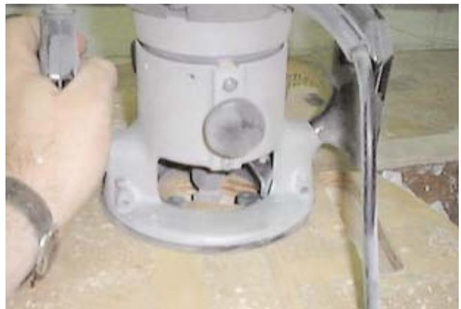
After the neck pocket is routed lay the neck in the neck pocket it should fit snug. Check the centerline to confirm it is lined up with the rest of the body routs. It's good to lay a long ruler down both sides of the neck and draw a line on the body. Hold the ruler against the sides of the neck from around the 15th fret tightly against the neck and draw the line make sure you hold both sides the same.
