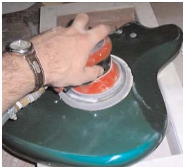
I use a palm sander with #800 dry on it and sand the area flat until all the shiny spots are gone, and the seam lines disappears. Then I use #1000 and #1500 wet, then buff the area. If you don't have a palm sander just use the #800 wet with a flat block to sand out the seams then follow the #1000 and #1500 paper and buff.
