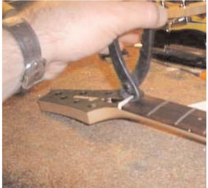
Then use a hammer and a short metal piece to pop the nut out. Lay the flat edge of the metal bar against the nut and give it a sharp tap with the hammer. The nut should come loose then lift the nut out of the slot. For Fender® style nuts that are bone, or graphite these can be tricky. The best way I have found to remove these nuts is to use a pair of end nippers that remove the frets to wiggle the nut until it becomes loose and then remove it.
