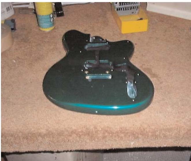
I use the buffing wheels because I have them, but you can get the same shine using a buffing compound that would be used on a car and just rubbing the scratches out. In the states I use a 3m compound and then I use a car polish called Macquires to bring the body to a high gloss.
