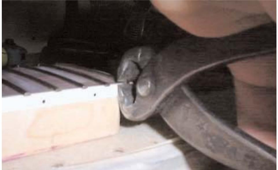
The next step is to cut the frets back with the end nippers, be careful not to lift the fret. So I tend to cut the frets from the side with the nippers, then I use a flat coarse file to file the fret ends back to the wood.
