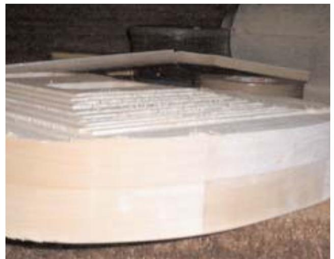
Once the step routing is finished you will see the basic shape of the arched top. From this point I use a round chisel to carve off the sharp edges.
