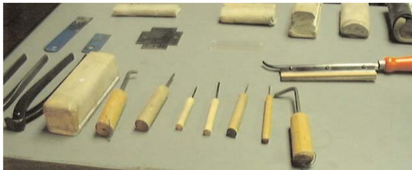
second they are easier to find on a crowded desk and best of all then can be setup on a work bench for easy access. To do this I just use a grinder to make the wrenches straight and drill into the dowel the correct size and super glue the wrench in. The upper left tools are hand made scrapers that I make from old hack saw blades. Next is my custom nut cutting template that
