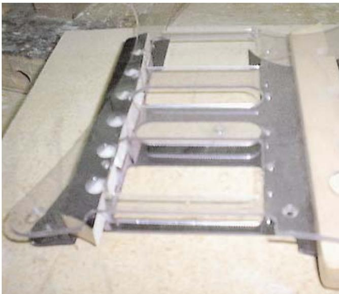
Make sure you raise the old pickguard above the new piece other wise there is no room for the bearing. Just drill out the other holes for the pots and if you have a 5way switch drill some small pilot holes where the lever will be and clean it up with a small file. I use the mill to do this for a one of a kind.
