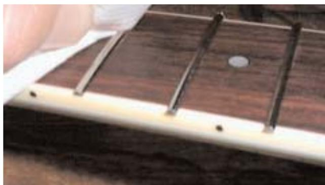
After all the frets are placed in the neck, again wipe the board down with the alcohol.
