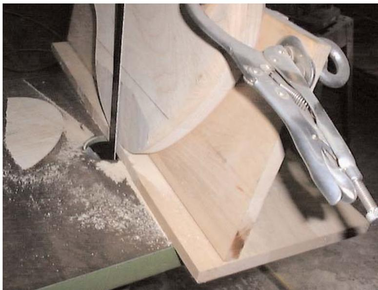
When I first started making bodies I would make the comfort cuts on the front and back by hand with a rasp. This worked fine, but everyone was different; I once saw this jig in a factory so I made one myself.
