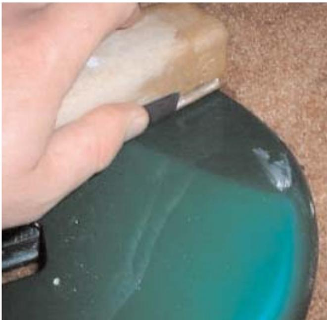
Wet sand the body in a back and forth motion with #1000 and #1500 to get the circle scratches out. The next step is I hand rub certain areas with a 3M Buffing Compound, but a car compound also works well. I do this to areas that are hard to get the buffer in on like some cutaway's or edges.
