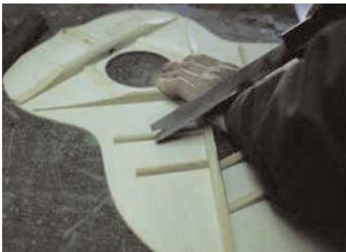
Scalloped braces are more common nowadays than they used to be. In the old days and still at Martin all scalloping is done by hand. Scalloping is when you shave the braces thinner to give the top better vibration with less stiffness caused by the braces. Asian factories have designed a machine that scallops all the braces simultaneously that they are cut to size and shape. Almost all factories now use some type of scalloped bracing.
