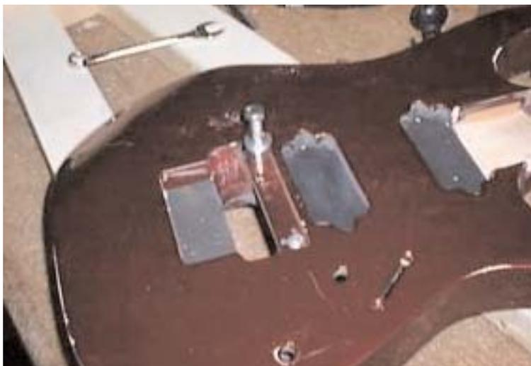
Next you will need a wooden dowel that is larger than the hole, If the hole is 10mm I use at least a 12mm dowel. Use the correct drill size for the new dowel and drill the insert area with the drill bit. Measure the depth that you drill and mark it on the dowel and cut the dowel to the exact length that you need. Remember most drill bits drill the center of the hole deeper than the sides so measure the depth at the side of the hole not the center.
