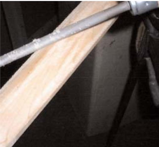
Now comes the fun part final shaping. First, rough out the fretboard radius so that when you hold the neck in you hand it feels natural then use round files to shape the actual necks back profile to the desired feel. Keep checking the shape with your hand and feel each area of the neck to verify it is what you want.
