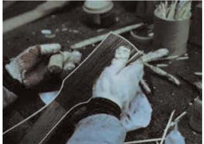
After the body is dry and removed from the side presses the binding channel is cut around the body using a modified router table; The body is then bound.
