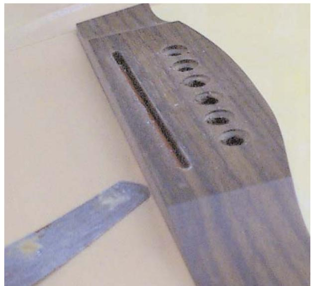
So what do I do today? Well if I will completely replace the bridge with a new one then I rout it off with a hand router. I made a simple bridge template that I double stick tape on the top, and I just use a standard hand router and slowly rout down the bridge until it is just a micro thin piece over the top and the last piece just peels off leaving the top perfect for the new bridge.
