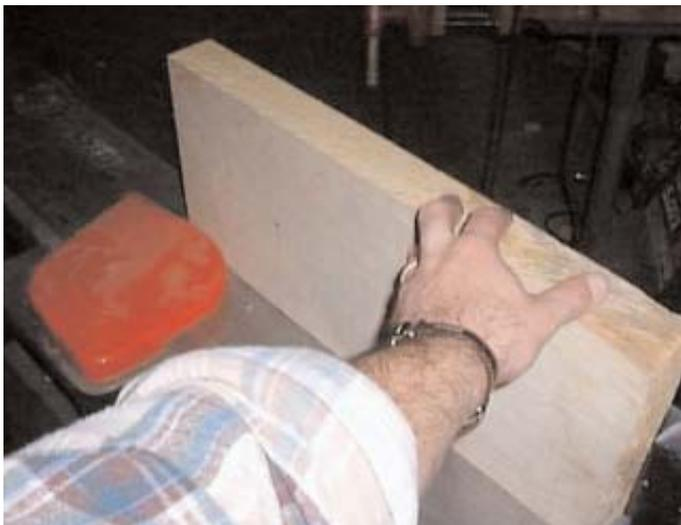
After the tracing use the jointer to get the sides of the wood ready for joining.
