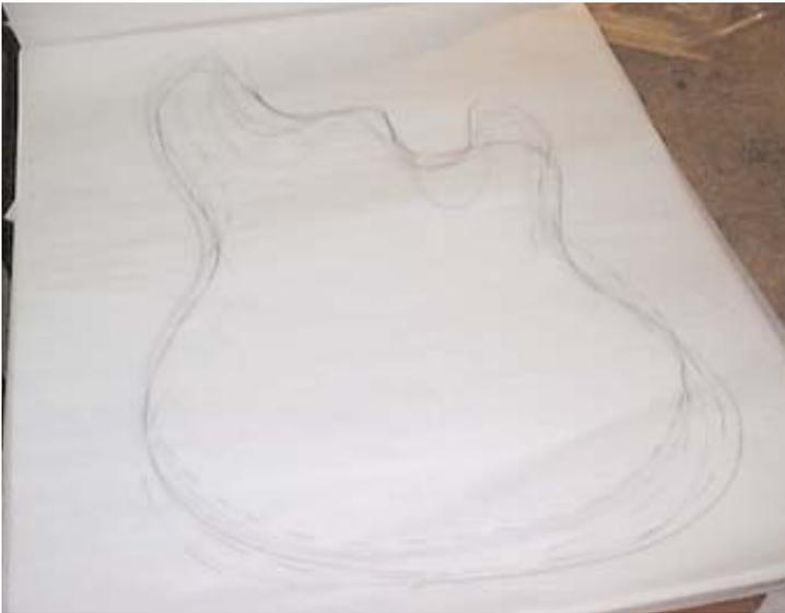
Now if the customer gave you a drawing, find the center of the drawing and make a line. If you are copying another guitar find the center and lay it on center with the neck pocket as a position guide and trace the body.
