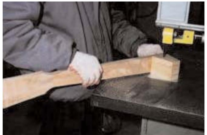
They have many different cutters and jigs for shaping all the parts of the neck. To keep the neck production consistent they have specially made cutters that have the shapes for the back of the neck and heel area, these machines are very high speed so they make large jigs to hold the material without standing too close to the blades.
