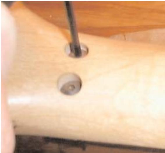
If the guitar has a locking tremolo make sure that the two bolts that hold the lock nut on are tight.
