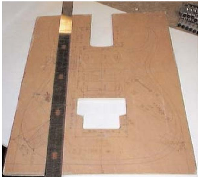
If I did not have a drill press I would first try to find one or if all else fails use a thick piece of scrap wood, Drill through it nice and straight and then put the drill bit through that piece of wood, line up the drill bit to the punched hole in the wood and use the scrap block as a straight guide to drill the hole.
