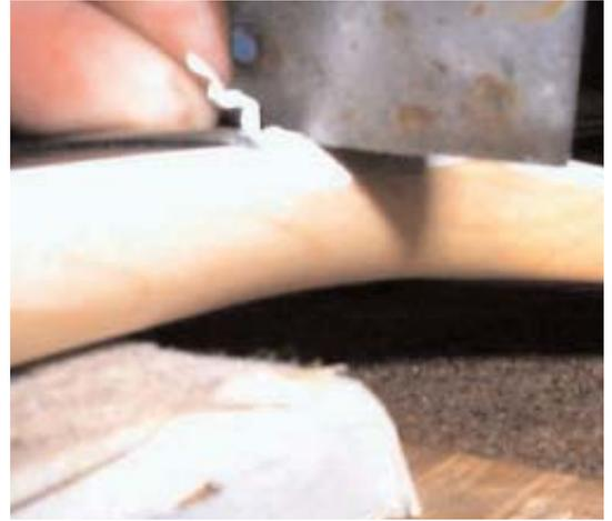
If the fretboard has binding I then scrape the binding using my scraper that was made from a ground down hack saw blade.
