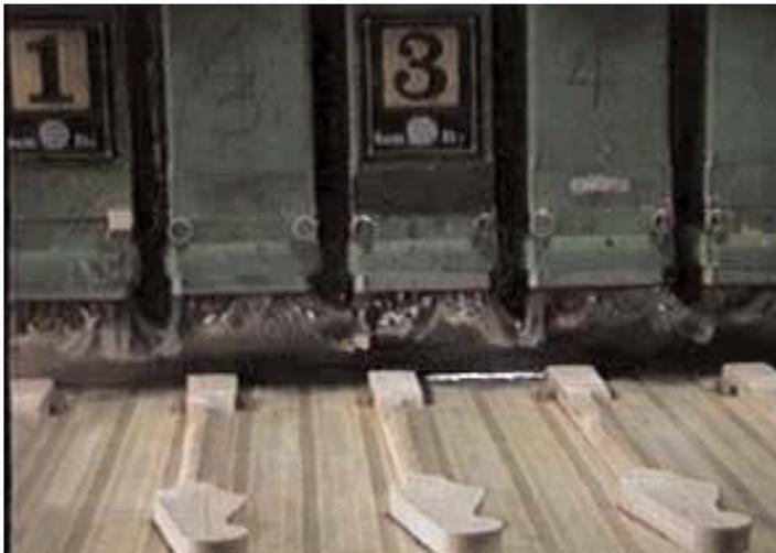
After the CNC rough shapes the necks, they still need a lot of handwork. First, they are moved to an area where the headstock and heel areas are shaped and the truss rod slots are cut.
