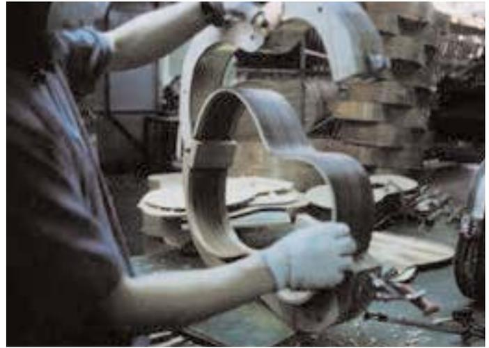
Before gluing the top on they cut the ends of the bracing. This could be done before they installed the braces but because it is much easier to keep accurate the length of the braces so they are flush with the sides of the body; this is important for the sound transfer to the top.
