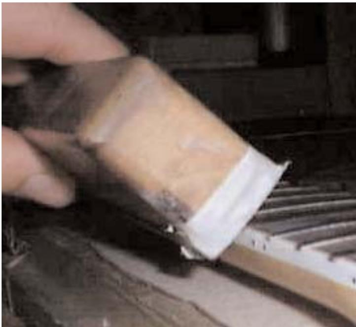
Take the glue and put it on a piece of wet sandpaper and use a toothpick. Take the glue and touch it on the top of the fretboard below the fret and watch in amazement as the air bubble disappears. Then use the #280 long block to sand the fret end back, Follow the same procedure as above to finish the frets.
