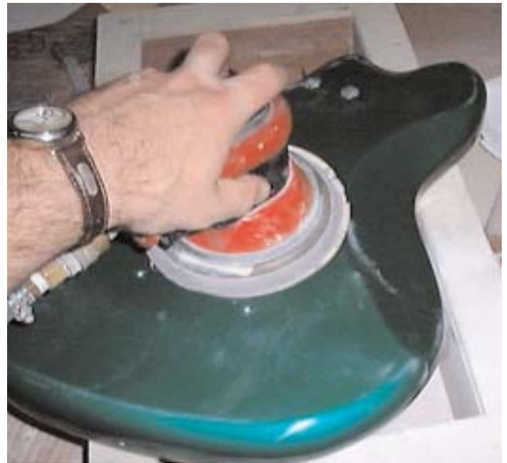
Once the body is sanded I use an up-right buffing wheel with a German Menza compound. First I use an abrasive wheel with the compound on it to get the fine sanding scratches out and then a second wheel that is just soft cotton to bring out the shine.
