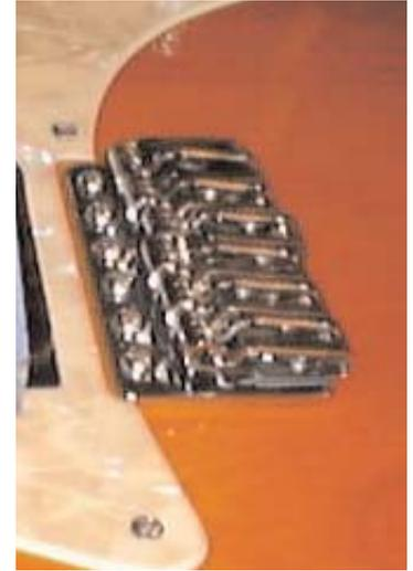
For locking tremolo bridges a big problem I have seen is that the inserts in the wood can become loose and move. To check this just look at the stud inserts in the wood when using the tremolo if they are moving, the guitar will not stay in tune also the action could change after using the bar. The correct way to fix this is to remove the metal insert, glue a dowel in the hole, re-drill it, and replace the insert.
