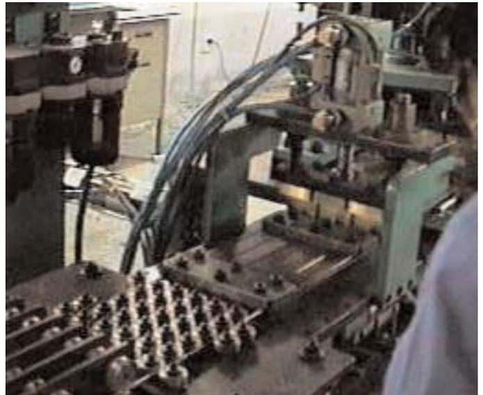
The frets are first hammered in manually, just to set them and then the frets are pressed in using an arbor press.
