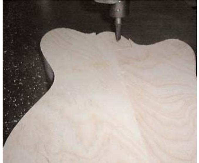
For example, if the binding is 2mm I use an 8mm pin with a 12mm bit this will rout a perfect 2mm channel for binding.
