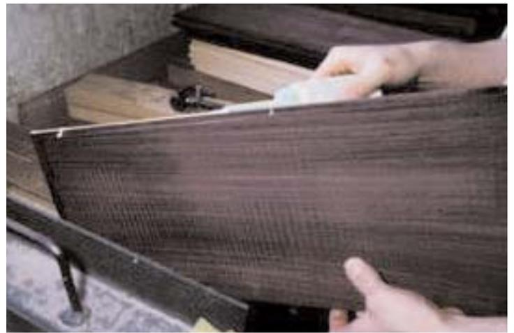
First, the wood is book-matched. Book matching is taking a piece of wood and splitting it down the center, then you open it up like a book and join the wood. The wood is laid flat on a table and two side clamps are closed on the wood, weights are laid on the joint to remove any flexing. The glue sets in about 30 minutes and takes 24 hours too completely dry before any production can begin.
