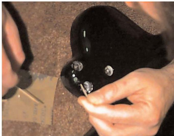
Take one drop! No more on a toothpick and place it in the edge of the crack so the glue runs under and in the chip. Don't use your fingers on this because super glue adheres to skin better than anything, Use the second tooth pickup with no glue on it to hold the chip in place while the glue dries.
