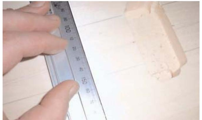
I will use a 12mm bit to rout so I measure every 12mm's and make another line. For the back by the bridge I want the arch to be less until after the bridge and then carve down, for this I will step rout 1mm depth every 12mm's until I reach the 6 mm depth than I will increase it 2mm every 12mm's.
