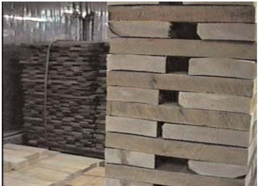
The woods are first sorted, cut to size, planed to the correct thickness and placed in a drying room to sit for a few days until the moisture content is stable.
