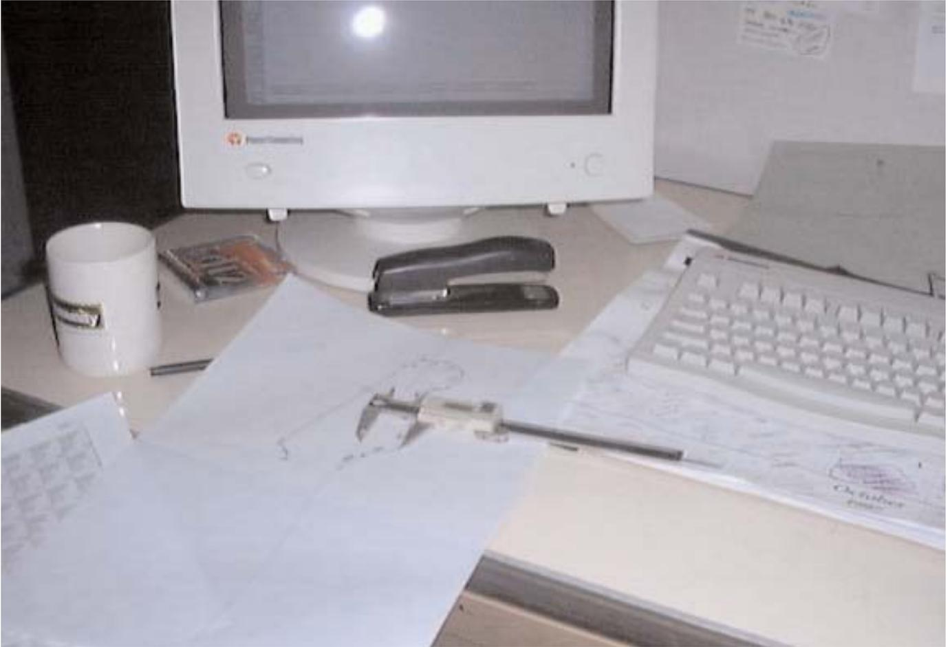
Take the graph paper and start with a centerline down the middle this will be 0 on the X-axis, Then trace the body or neck layout on center. After the body or necks are traced onto the paper we use the radius gauges all around the body to check each arcs location and radius. Mark the points of the beginning of the radius and the end of the radius as it follows the gauge.
