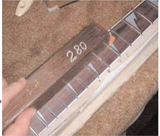
Sand the frets back and forth until all the marker is removed and look to see whether any marker remains in the fret grooves that were caused by playing. If so continue to sand with the long blocks to remove these dents don't concentrate in just one area but sand long strokes to keep the frets even. Check the line over the top of each fret; this will show where any high spots are.
