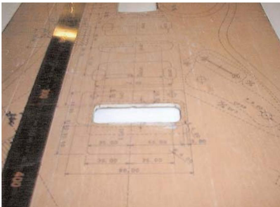
Always start from center, so make a centerline down the middle using a straight edge. This is the most important part. Use the scribe to mark a centerline into the material, you will need this when aligning the template to the surface for routing.
