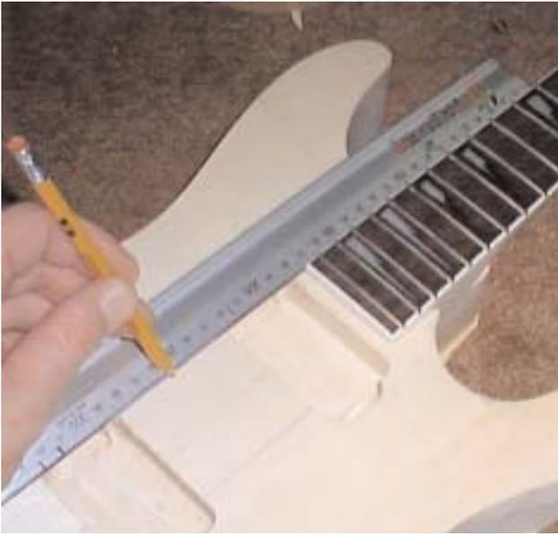
on the top. I usually like to keep the pickup area as well as the bridge location on a flat surface. I will start carving after these routs. For this example I will make a 12mm arched top from the center. I want the arch to be fairly steep so I will step rout 2mm at a time.
