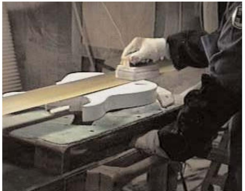
When the bodies are completely wet sanded to #1000 they are first buffed on a buffing machine, using a liquid compound that is brushed on the top and back. The table moves back and forth and side by side. This machine buffs the top and back and the final buffing of the sides is finished on a buffing wheel by hand.
