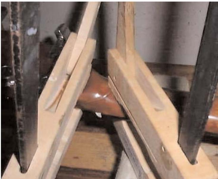
Don't worry about the height yet we will file and sand them after the glue dries. If the neck has a finish; hopefully, it has a sunburst right at the area of the repair. Then I will blow the burst in and refinish the whole neck.
