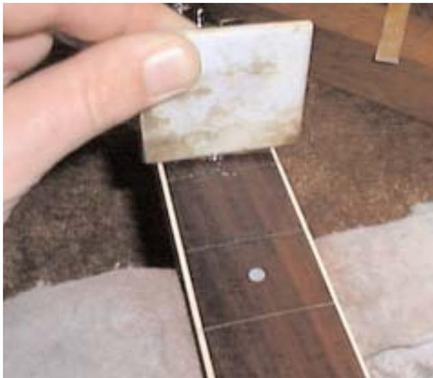
I use a modified piece of wood that has half the slot depth sanded away on it. I use this to clean out the epoxy in the slots half way down; this is so that when I place the frets in, the excess epoxy only comes up to the top of the slot and none comes out and onto the fretboard.
