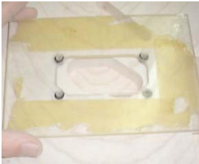
Lay the humbucking templates over the pickups and rout them as above to the correct depth needed for the pickup you are putting in. usually around 18mm's deep for the main part of the pickup.
