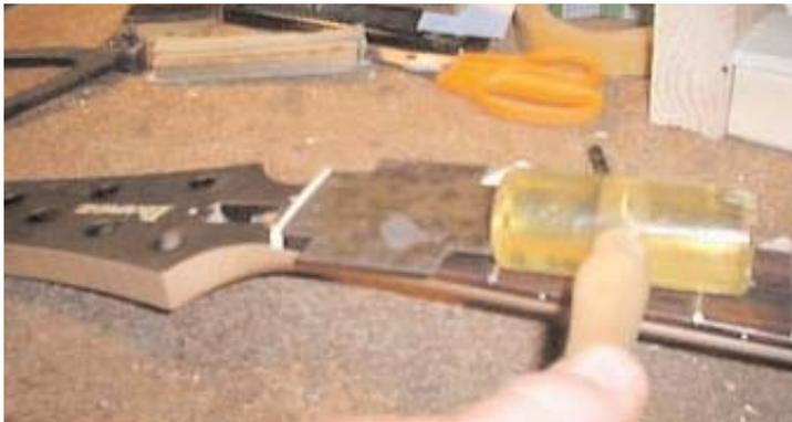
On a blank style nut I use a small metal bar to pop off the nut. With a Fender® style nut I try to wiggle it out with a pair of dull fret nippers, be careful you can easily take the wood with it. I read somewhere to saw the nut in half-long ways down the center. I tried this and it worked however, I always like to keep the original nut intact for at least marking the nut slots for the new nut.
