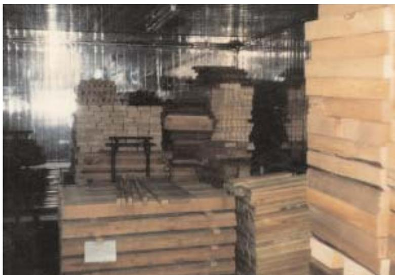
The woods are delivered and stacked up in the building to be cut, planed and joined; some of the smallest factories purchase the wood already joined to size.
