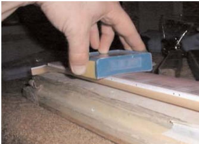
After the frets are removed and the board is sanded to the proper radius. We are ready for fretting. First figure out the size and depth of the new fret by using a dial or digital caliper. Use the manufactures specs with caution, I have had many problems with Dunlop frets tang and stud width for many years. Measure the tang and stud width as well as the depth of the tang.
