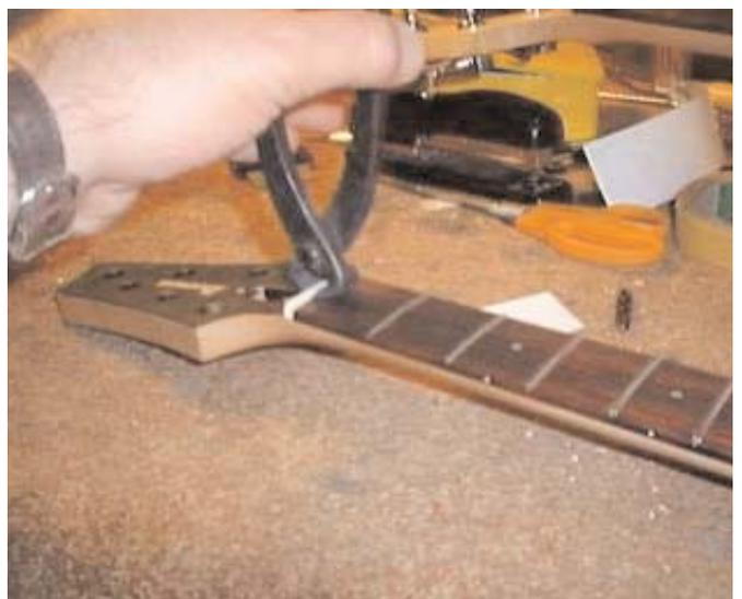
To install a new nut measure the nut slot and nut material. Cut and shape the nut material to the exact size of the nut slot before gluing it in. I use super glue to mount the nut, but you can use white glue if you want.
