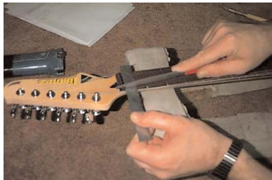
Again, different bridges have different ways of setting the action. A locking tremolo and a Gibson® style bridge will have two studs at either side that raise or lower the bridge. Strat style tremolos have the individual height adjustment for each string, and some modern tremolos will have both.
