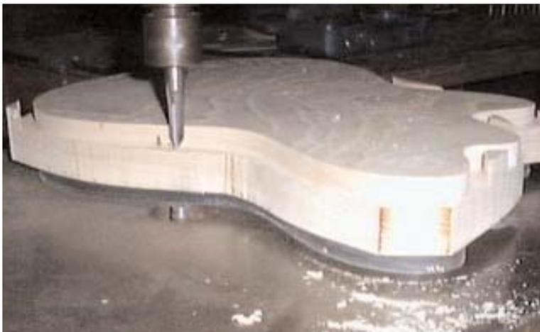
The next step for me is to take the body to the pin router and rout the bodies shape and all the front and back routs for the pickups, tremolo and electronics.
