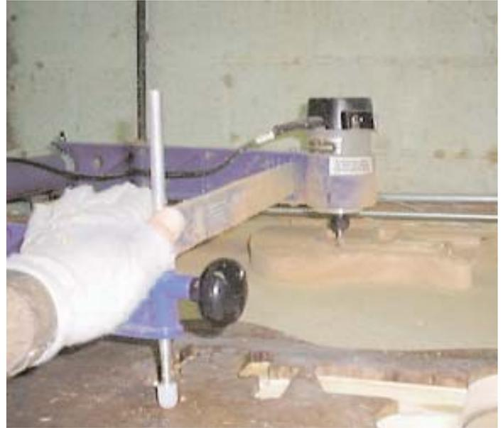
Once everything is lined up and depending on the wood I set the depth of the router bit higher than the actual final cuts. ( The depth I go on each pass depends on the wood. harder wood not so deep passes but a softer wood like spruce you can go fairly deep. This is actually gutting the wood. The pin is easily adjustable. Once it is set I go back and forth until the basic arch is carved.
