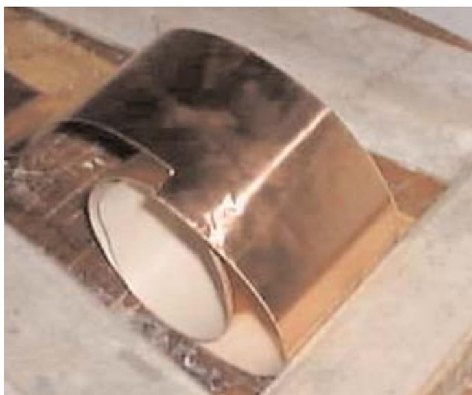
wires, and no shield could pickup allot of noise through the drilled area that the wire runs through. This is next to impossible to use tape in so I pour the shielding paint in the hole to seal it. If I really want the guitar to be quiet, I replace the two wires with a shielded two-conductor wire.
