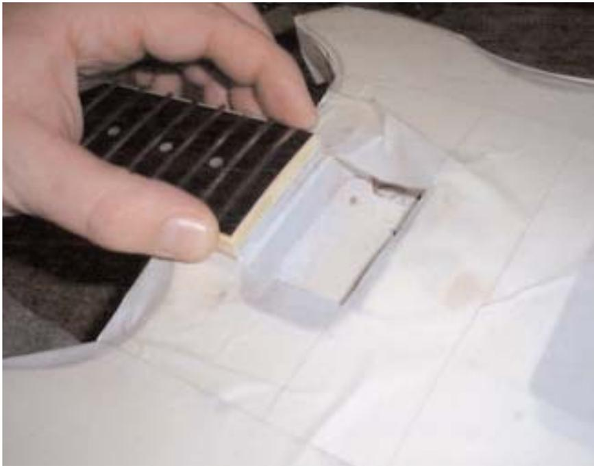
Each fret is placed in the slot to check that it fits well, and then I carefully remove it, on some boards like ebony I will use some Lemon oil on the wood before I put the frets in so that when I pull them out the wood does not chip. If you use the lemon oil only use a little and make sure it is only on the top of the fretboard and none gets in the fret slot.
