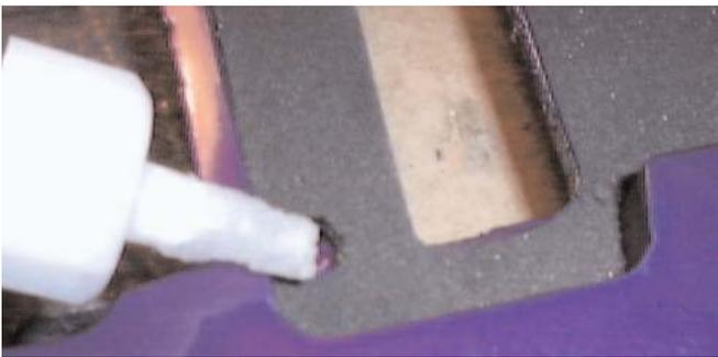
But, this is not always possible at home so what I do is take the bridge off, push the insert all the way in the hole and take super glue and pour it around the outside of the insert. This is not actually gluing the metal to the wood, but the wood absorbs the super glue and when the glue hardens the wood become much stronger.
