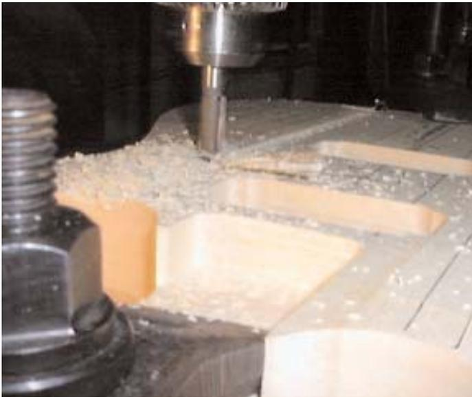
Continue milling each line to the proper depth.
