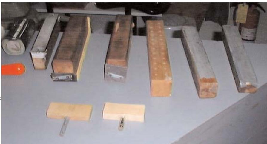
This is a collection of tools I made for set up. Just Allen wrenches set in dowel rods. First, they are much easier to use than a standard angled wrenches,
