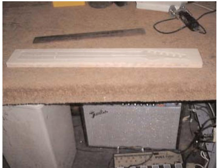
Next I get the wood ready; I have found that the best way to make a neck is to start from the exact thickness wood needed. For example, if the neck at its thickest part is 25mm (At the neck pocket) and I will use a 4mm thick fretboard I will plane the wood to 21mm before I even start making the neck, once the neck is glued up I don't want to remove any extra wood just shape the back and it's done.
