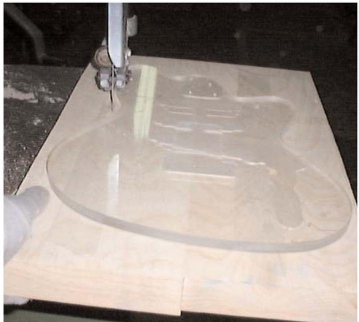
Once the body was cut, the edges were rough and I also usually stay on the outside of the bodyline when cutting because I don't like to make a mistake. I have seen many people that can cut exactly on the line, but it is too much of a chance to make a mistake.
