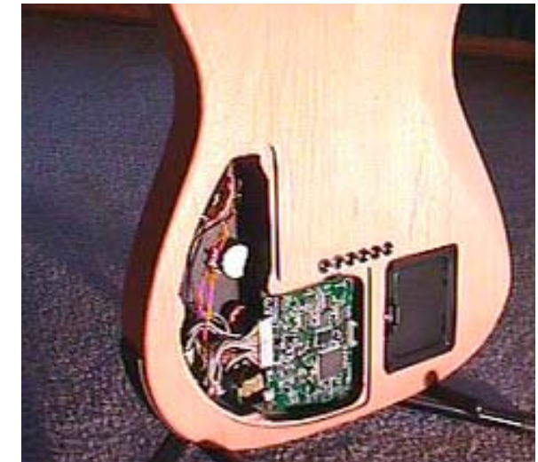
Fig.: 4.4: Line 6 electronics as mounted on the back of the guitar.
