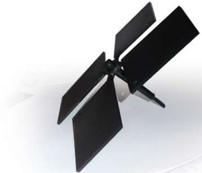
Fig. 3.27: Four parts in one cold runner mold.
