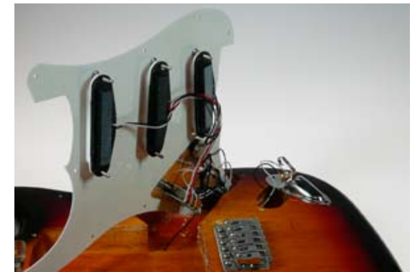
Fig. 3.11: Photo of the electronics, the pickguard and the output jack.
