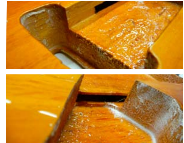
Fig. 3.4: Photos of the milled cavities in the body.
