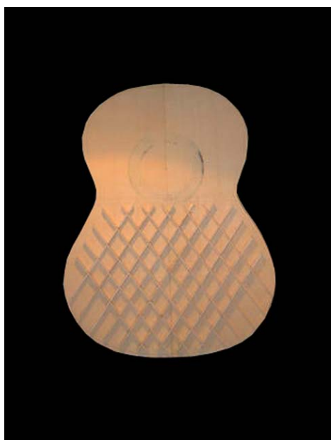
Figure 4.7 The lattice-braced soundboard of the Cleveland guitar featured in figure 4.6.
