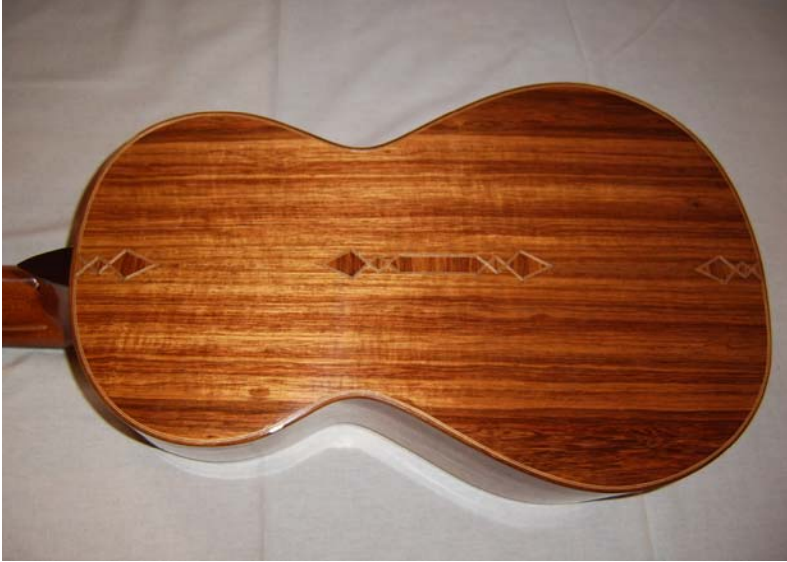
Figure 3.4 Ornamental inlays in the Kiaat back of a Pickard instrument.
