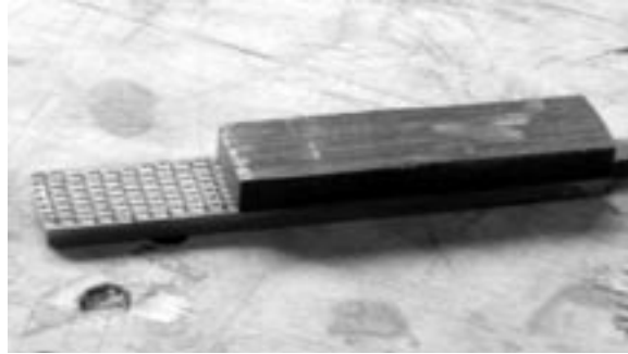
A rasp used to form the edge height on carved plates
