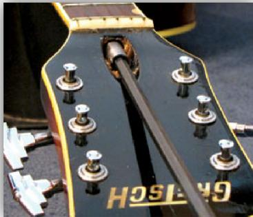
The location varies on different guitars but is usually located at the end of the neck or behind a plate on the head. If your neck is bowed forward, you will want to tighten the nut to bend the neck backwards. If your neck is back-bowed, you will want to loosen the nut which will allow the neck to straighten or bow forward. As a rule of thumb, never adjust the truss rod more than 1/8<sup>th</sup> turn at a time. Over
