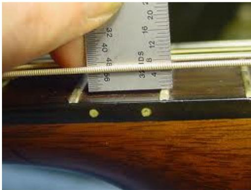
above the fret board are known as “High-action” the opposite goes for strings that are set low. The Action of a guitar is important when determining its playability. If the action is too low, then it can cause string buzzing. If the action is too high then it will start to become uncomfortable and difficult to play. So it’s good to find a median where it is high enough to not cause
