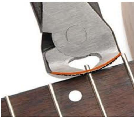
**Nip the Fret Ends-**After the glue has dried, you can take a pair of end nippers and cut off the edges of the frets that are hanging off the sides. After they are nipped off, you should take a file and smooth down the edges. Make sure to file downwards on the side of the board. If you file upward then you risk loosening your frets.
