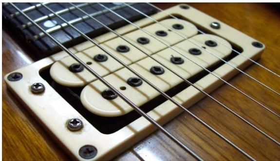
“float” in place. The height can be adjusted by tightening or loosening the mounting screws, and thus also allows the tone quality to be adjusted.
