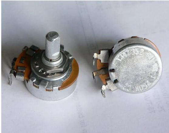
One of the parts commonly mentioned on electric guitars are the pots, but what exactly is a pot? Pot is actually short for potentiometer, a small device that controls the flow of electric current making it basically a glorified resistor. A guitar will usually have 2 pots; one is for volume and the other for tone. On the bottom of each pot
