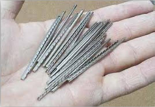
Fret wires are commonly made out of nickel and stainless steel, although they can be made out of several kinds of materials. Stainless steel is much denser than nickel which helps prevent wear. On the other hand stainless steel is much harder to install than nickel due to its density. Nickel is often recommended for the average player.
