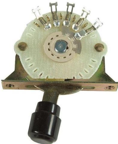
A pickup selector is a simple electronic switch that is hardwired to both the guitar pickups and eventually the guitar jack. When the switch is flipped in a direction, the switch connects the lugs wired to the pickups and the jack completing the circuit. This is how the pickups are selected. While one or a combination of pickups is selected, the other pickups are deselected by the same means.
