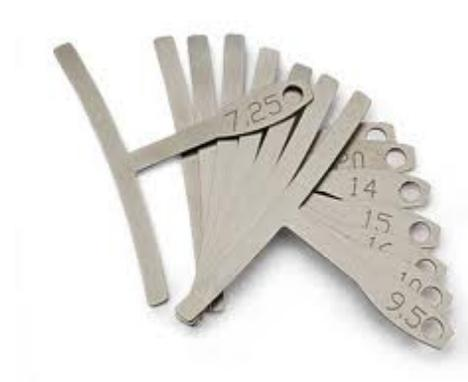
Fret boards have a slight curve to them known as the radius and this will have to be measured if you want to install new fret wire. To measure the radius, you will have to take the strings off and place a radius gauge against the board. Turn the gauge until you don't see any light coming through when you have the gauge placed on the board.
