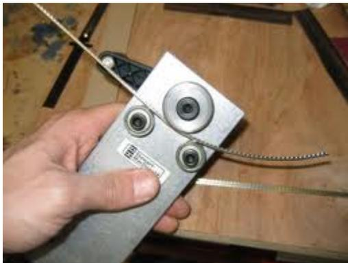
Fret wire will usually come in 1 or 2 foot sections, although they can be bought pre-cut. This fret wire will initially be straight but to fit it on to your guitar, you will have to bend it to the radius of your fret board. You can use a fret wire bender to correctly bend it to fit your fret board
