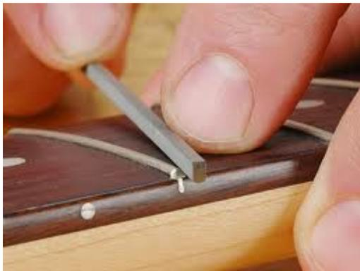
**Bevel the Edges-**To make your fret rounded on the edges you can use a fret bevel. Use a 35 degree bevel to get a 35 degree angle around the edge of the fret. Beveling will usually leave burrs, so use a three-cornered file to remove the burr. After the burr has been removed, sand the edge with a 320-grit, 600-grit, 800-grit, and 1,000-grit sandpaper.
