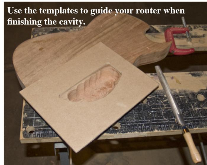
**Use the templates to guide your router when finishing the cavity.**
