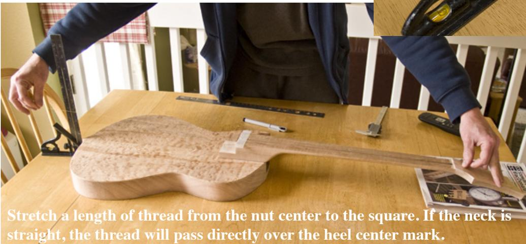
Stretch a length of thread from the nut center to the square. If the neck is straight, the thread will pass directly over the heel center mark.
