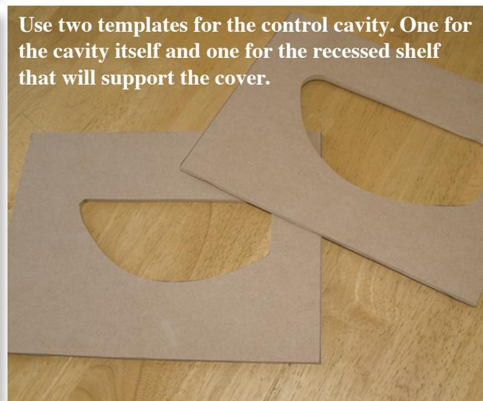
**Use two templates for the control cavity. One for the cavity itself and one for the recessed shelf that will support the cover.**
