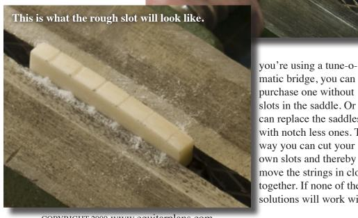
matic bridge, you can purchase one without slots in the saddle. Or you can replace the saddles with notch less ones. That way you can cut your own slots and thereby move the strings in closer together. If none of these solutions will work with
