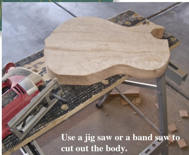
**Use a jig saw or a band saw to cut out the body.**
