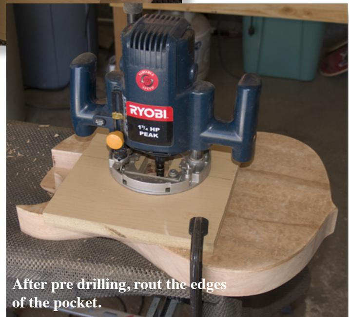
**After pre drilling, rout the edges of the pocket.**
