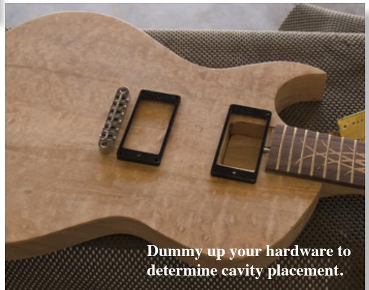
Dummy up your hardware to determine cavity placement.
