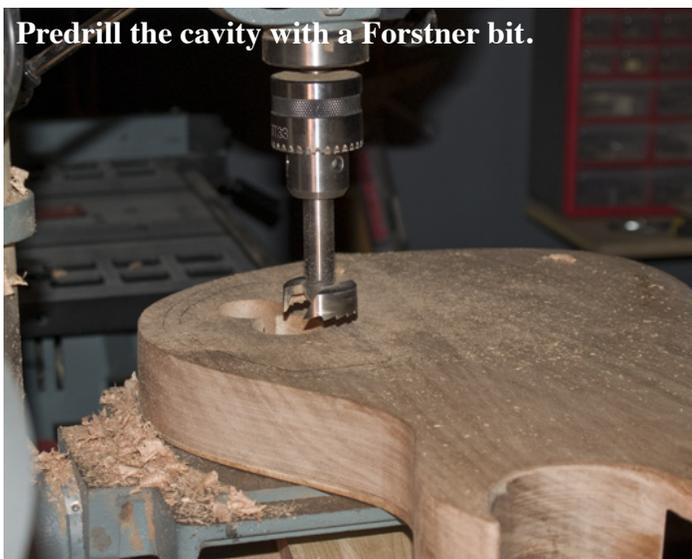
**Predrill the cavity with a Forstner bit.**
