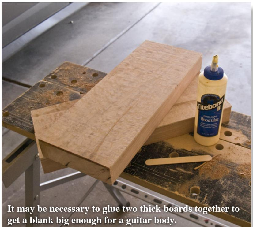
**It may be necessary to glue two thick boards together to get a blank big enough for a guitar body.**
